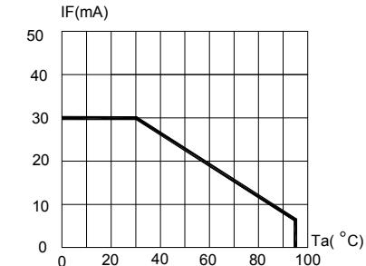
FIG.5 MAXIMUM FORWARD DC CURRENT
