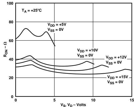
Figure 4.  $R_{ON}$  as a Function of  $V_D$  ( $V_S$ ): Single Supply Voltage
