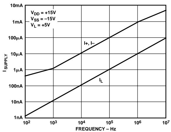
Figure 7. Supply Current vs. Input Switching Frequency
