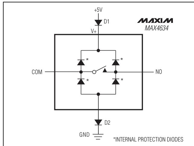
Figure 1. Overvoltage Protection Using External Blocking Diodes
