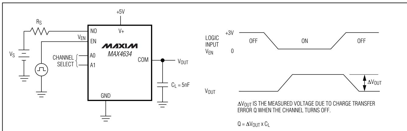
Figure 4. Charge Injection
