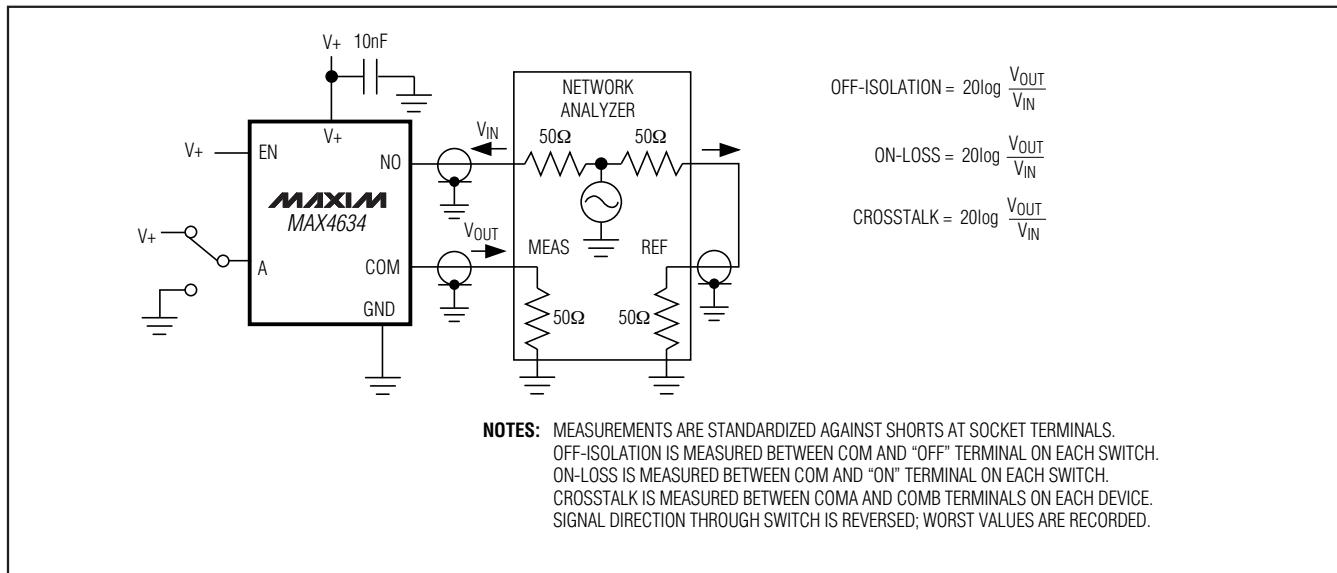
Figure 5. Off-Isolation/On-Channel Bandwidth
