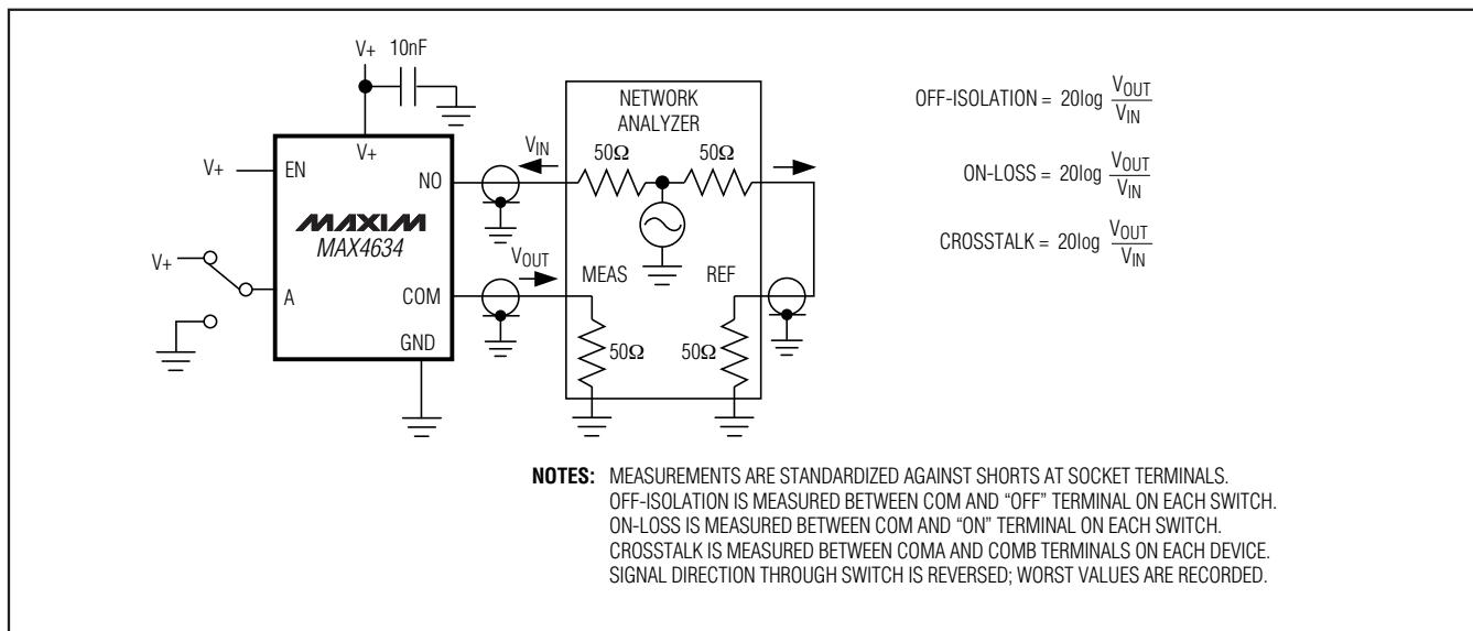
Figure 5. Off-Isolation/On-Channel Bandwidth
