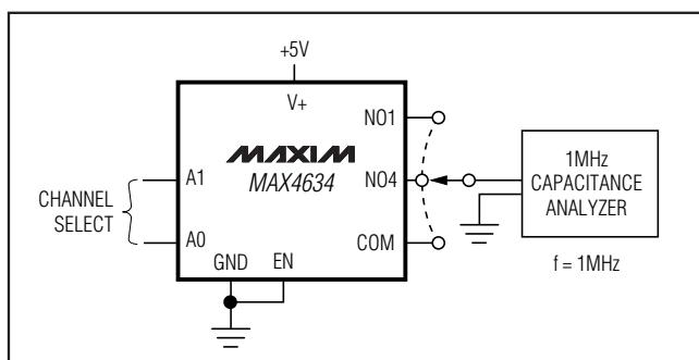
Figure 6. Channel Off/On-Capacitance
