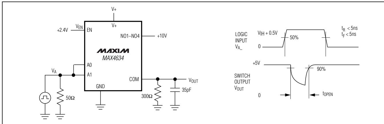
Figure 3. Break-Before-Make Interval
