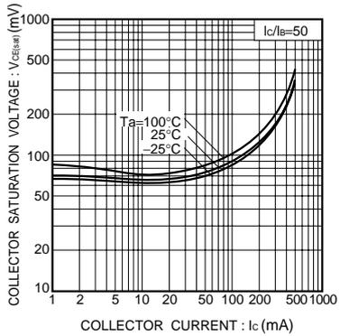
Fig.7 Collector-emitter saturation voltage vs. collector current ( IV )
