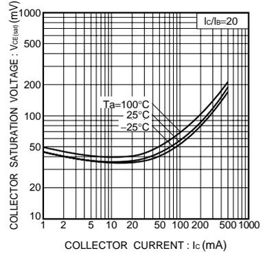
Fig.6 Collector-emitter saturation voltage vs. collector current ( III )
