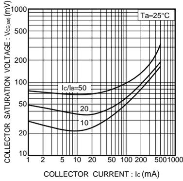
Fig.4 Collector-emitter saturation voltage vs. collector current ( I )
