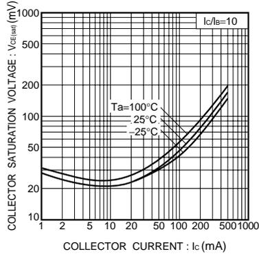
Fig.5 Collector-emitter saturation voltage vs. collector current ( II )
