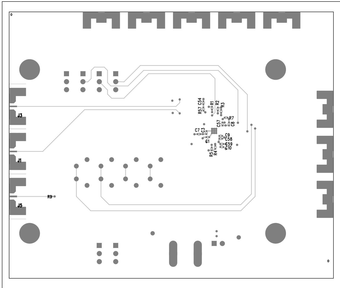
Figure 7. MAX3679A EV Kit Assembly Drawing—Bottom Side
