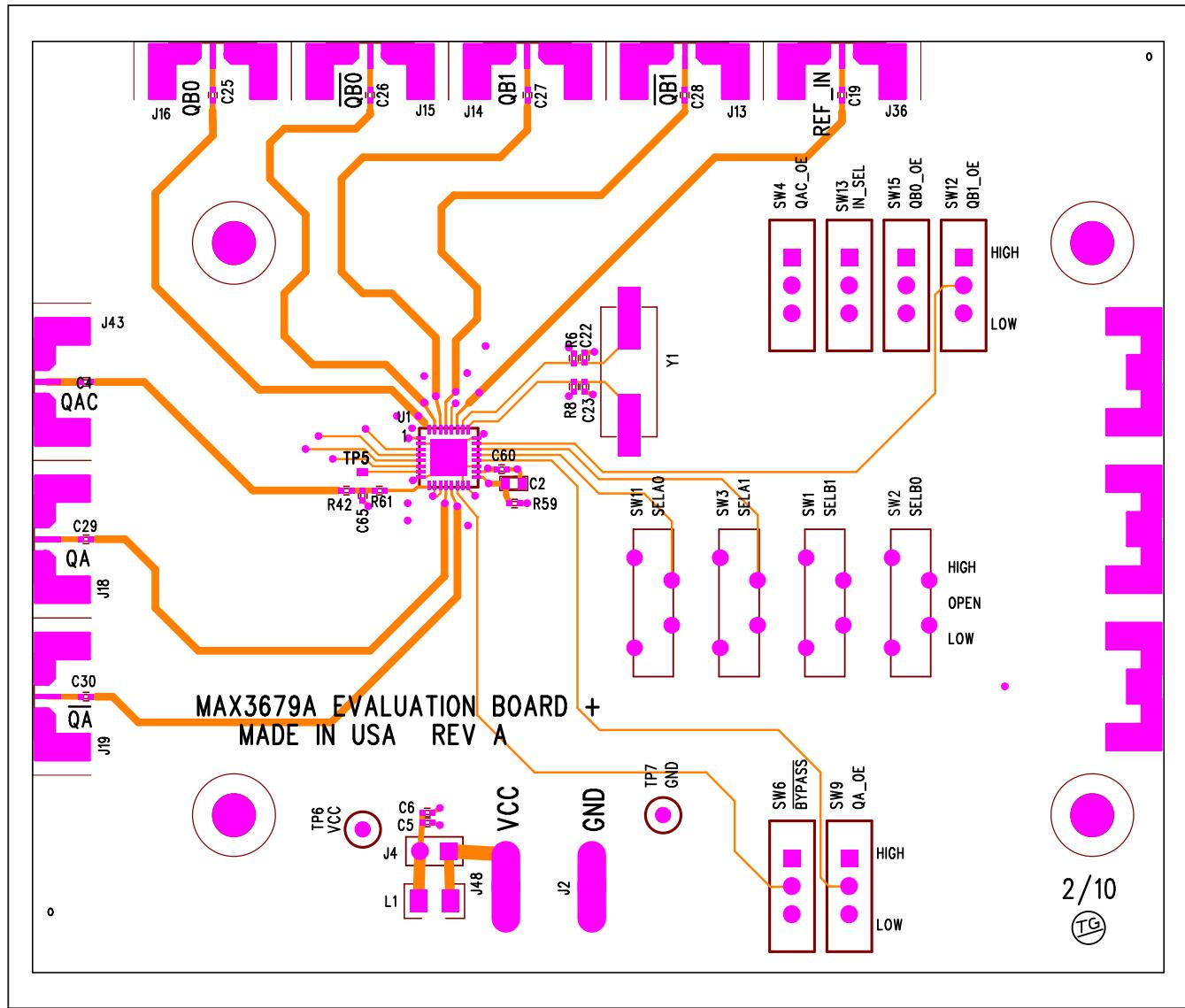
Figure 2. MAX3679A EV Kit Assembly Drawing—Top Side
