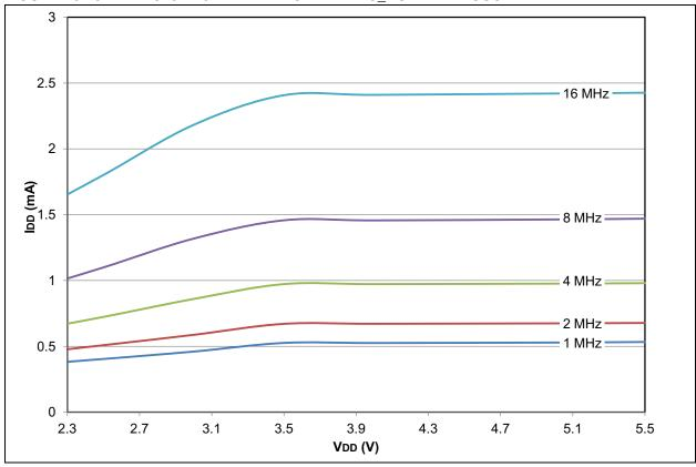
FIGURE 28-29: PIC18F2X/4XK22 MAXIMUM IDD: RC\_RUN HF-INTOSC
