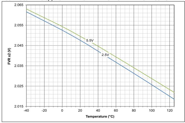
FIGURE 28-97: PIC18(L)F2X/4XK22 TYPICAL FIXED VOLTAGE REFERENCE 2x OUTPUT
