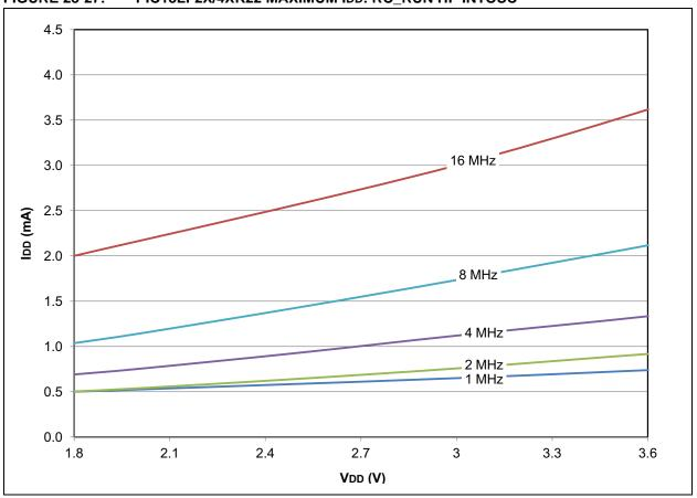
FIGURE 28-28: PIC18F2X/4XK22 TYPICAL IDD: RC\_RUN HF-INTOSC
