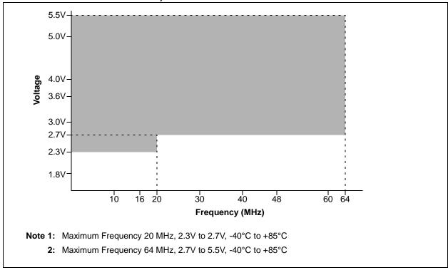
FIGURE 27-4: PIC18F2X/4XK22 FAMILY VOLTAGE-FREQUENCY GRAPH (EXTENDED TEMPERATURE)
