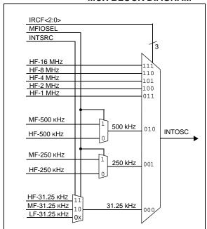
FIGURE 2-3: PLL\_SELECT BLOCK DIAGRAM
