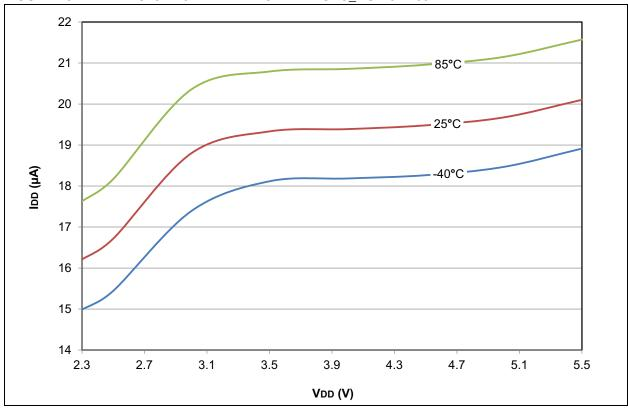
FIGURE 28-75: PIC18F2X/4XK22 MAXIMUM IDD: SEC\_RUN 32.768 kHz
