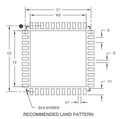
Units MILLIMETERS **Dimension Limits** MIN NOM MAX Contact Pitch 0.65 BSC Ε Optional Center Pad Width W2 6.80 Optional Center Pad Length T2 6.80 Contact Pad Spacing C1 8.00 Contact Pad Spacing C2 8.00 Contact Pad Width (X44) X1 0.35 Contact Pad Length (X44) Y1 0.80 0.25 Distance Between Pads G
