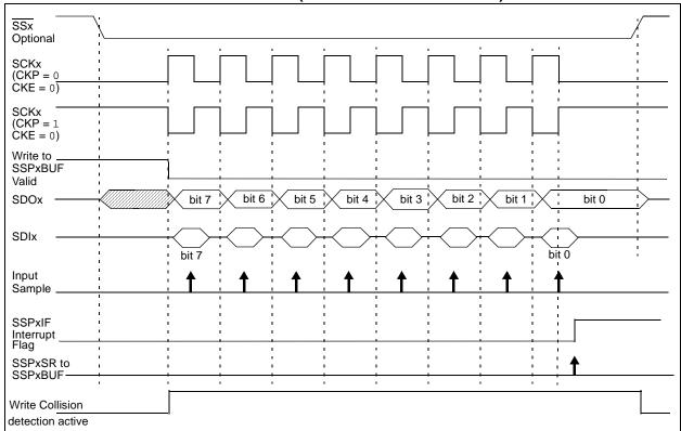
FIGURE 15-10: SPI MODE WAVEFORM (SLAVE MODE WITH CKE = 1)
