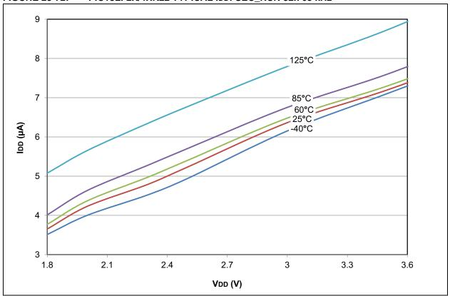
FIGURE 28-73: PIC18LF2X/4XK22 MAXIMUM IDD: SEC\_RUN 32.768 kHz
