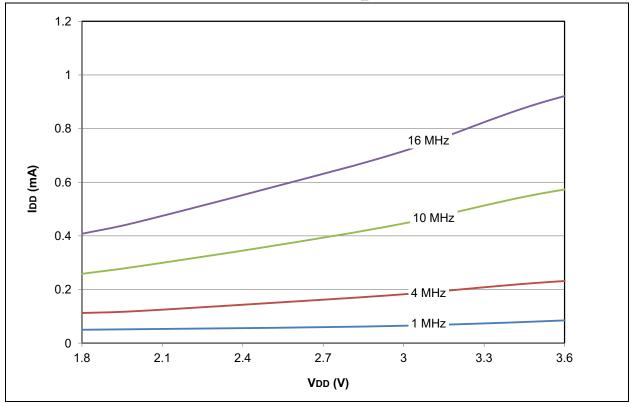
FIGURE 28-62: PIC18F2X/4XK22 TYPICAL IDD: PRI\_IDLE EC MEDIUM POWER 8.0 16 MHz 0.7 0.6 0.5 10 MHz loo (mA) 0.4 0.3 4 MHz -0.2 1 MHz 0.1 0 2.3 2.7 3.1 3.5 3.9 4.3 4.7 5.1 5.5
