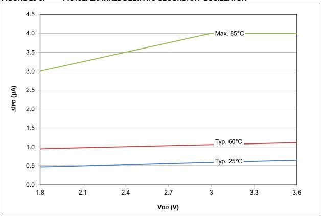
FIGURE 28-10: PIC18F2X/4XK22 DELTA IPD SECONDARY OSCILLATOR
