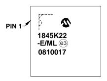
44-Lead TQFP (10x10x1 mm)
