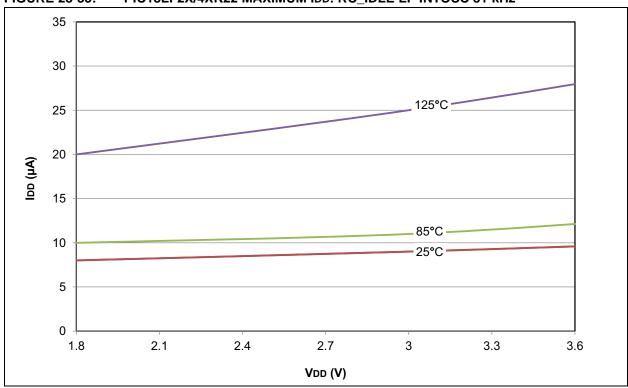
FIGURE 28-36: PIC18F2X/4XK22 TYPICAL IDD: RC\_IDLE LF-INTOSC 31 kHz
