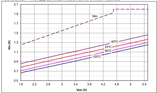
FIGURE 28-83: PIC18(L)F2X/4XK22 SCHMITT TRIGGER BUFFER INPUT HIGH VOLTAGE
