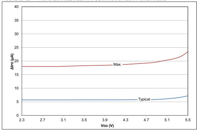
FIGURE 28-13: PIC18LF2X/4XK22 DELTA IPD COMPARATOR HIGH-POWER MODE
