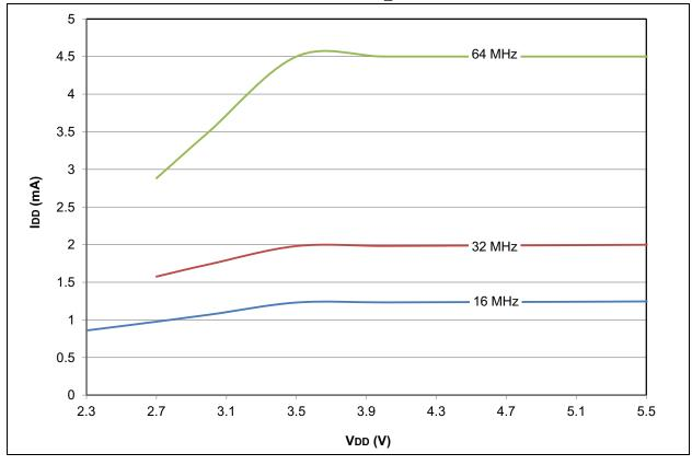
FIGURE 28-48: PIC18LF2X/4XK22 TYPICAL IDD: PRI\_RUN EC MEDIUM POWER
