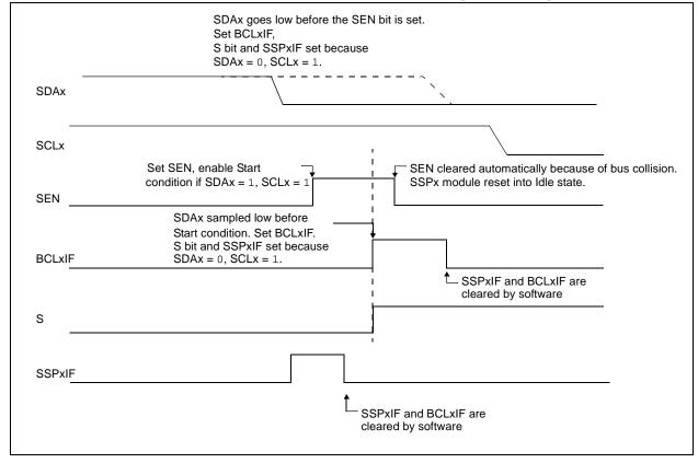
FIGURE 15-34: BUS COLLISION DURING START CONDITION (SCLx = 0)
