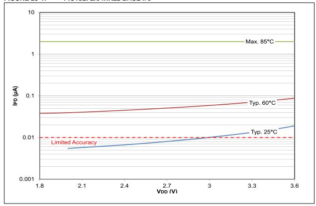
FIGURE 28-2: PIC18F2X/4XK22 BASE IPD
