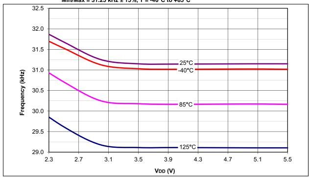
FIGURE 28-103: PIC18LF2X/4XK22 TYPICAL LF-INTOSC FREQUENCY vs. TEMPERATURE Min/Max = 31.25 kHz ± 15%, T = -40°C to +85°C
