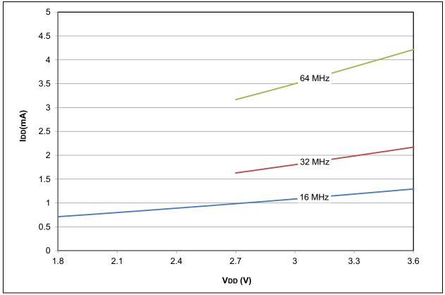
FIGURE 28-46: PIC18F2X/4XK22 TYPICAL IDD: RC\_IDLE HF-INTOSC with PLL
