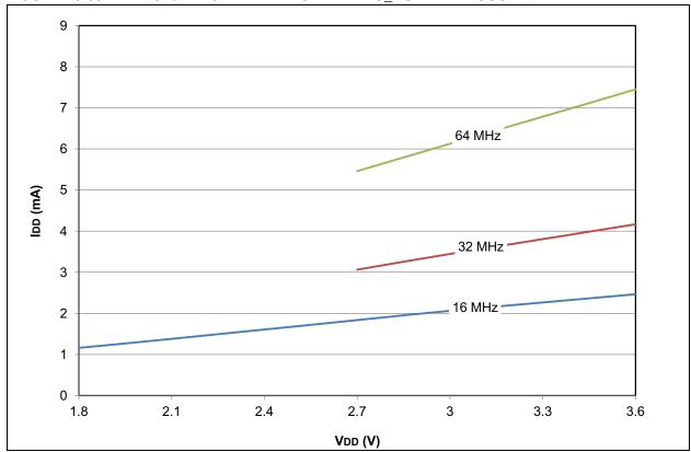
FIGURE 28-31: PIC18LF2X/4XK22 MAXIMUM IDD: RC\_RUN HF-INTOSC with PLL
