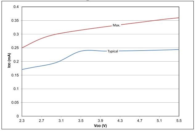
FIGURE 28-26: PIC18LF2X/4XK22 TYPICAL IDD: RC\_RUN HF-INTOSC
