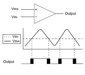
**Note:** The black areas of the output of the comparator represents the uncertainty due to input offsets and response time.
