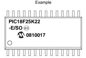
28-Lead SSOP (5.30 mm)
