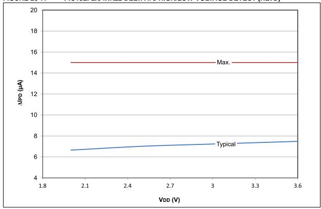
FIGURE 28-8: PIC18F2X/4XK22 DELTA IPD HIGH/LOW-VOLTAGE DETECT (HLVD)
