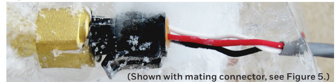
Figure 2. PX3 Series External Freeze/Thaw Resistance
