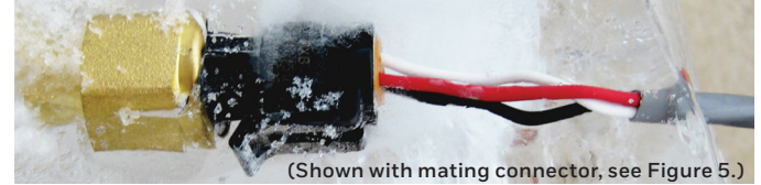
Figure 2. PX3 Series External Freeze/Thaw Resistance
