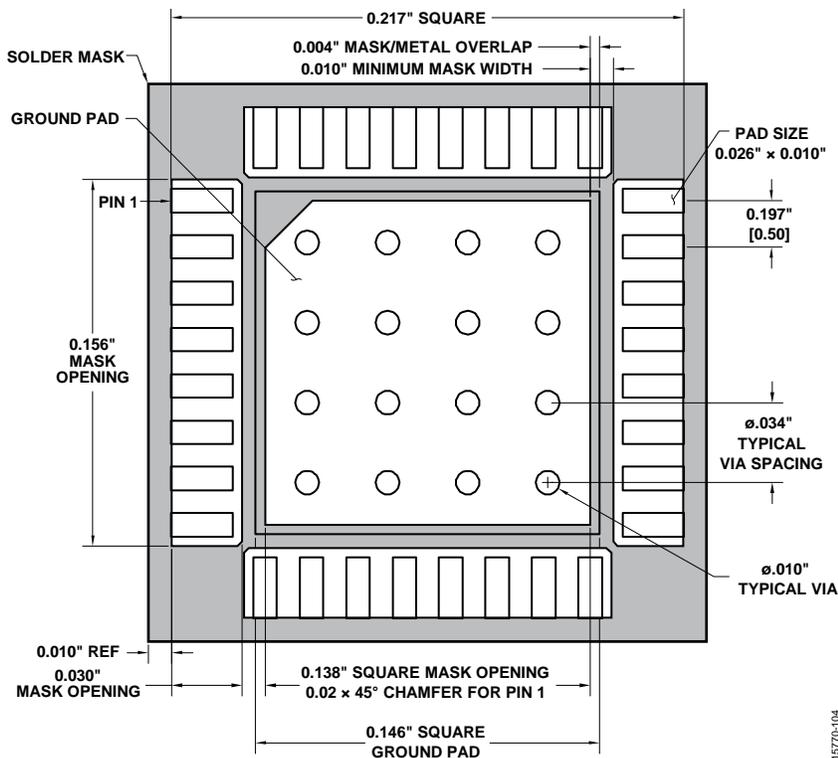
Figure 60. PCB Land Pattern Footprint of the ADMV1009-EVALZ
