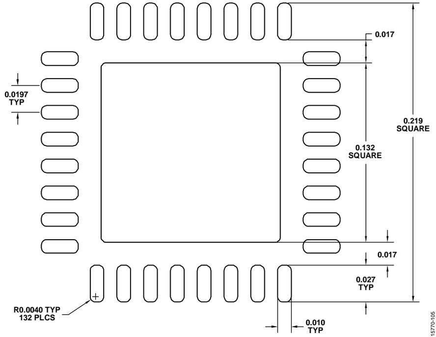
Figure 61. Solder Paste Stencil of the [ADMV1009-EVALZ](#)
