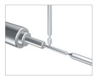
Precise Product Measurement Vacuum-retracting Sensor Heads enable post-processing measurements to be automated.
