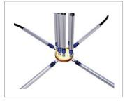
Small Parts Measurement Multi-contact Sensor Heads can be used to precisely measure all the dimensions of small parts at the same time.
