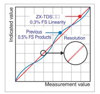
The long-stroke ZX-TDS04T $\square$  (4-mm measurement range) achieves high-precision measurement with the industry's top class of resolution (0.1  $\mu m$ ) and linearity of 0.3 FS max.
