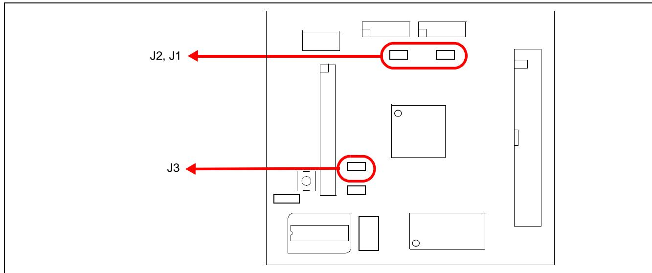
Figure 3-2: Configuration Jumper Locations (J1, J2, J3)
