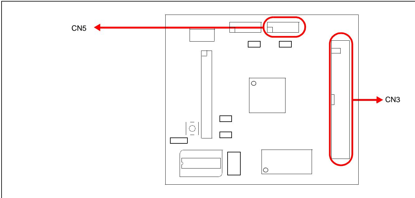
Figure 4-4: LCD Panel Connectors Location (CN3, CN5)
