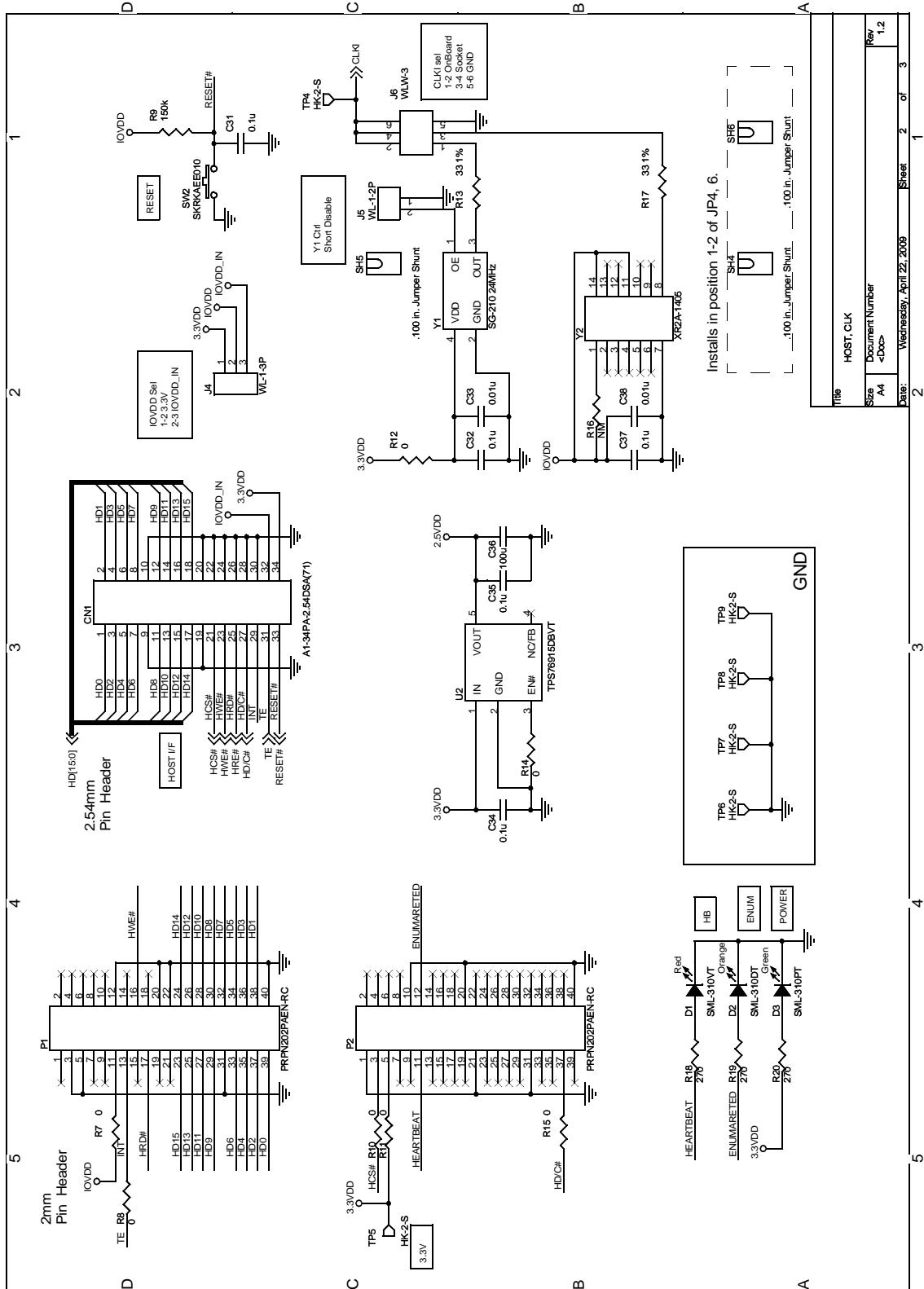
Figure 6-2: S5U13517P00C100 Schematic Diagram (2 of 3)
