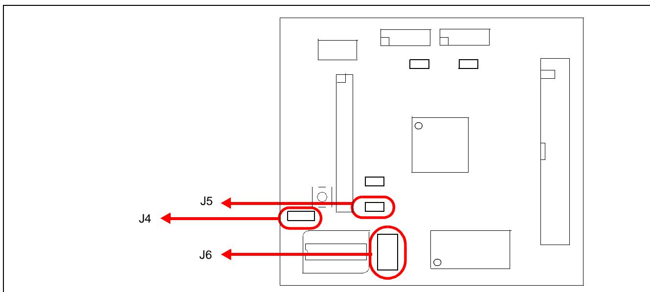
Figure 3-3: Configuration Jumper Location (J4, J5, J6)
