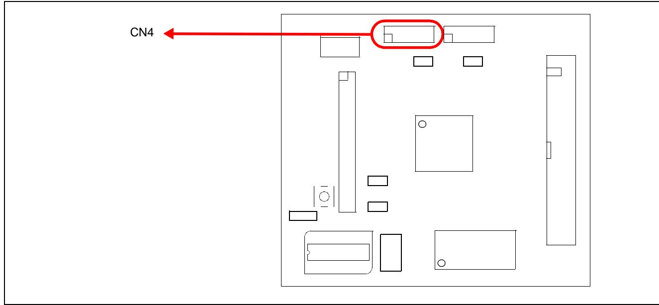
Figure 4-5: GPIO and PWM Connector Location (CN4)
