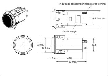
Note: Use a panel thickness of 0.5 mm for tab terminals #110 and solder terminals.
