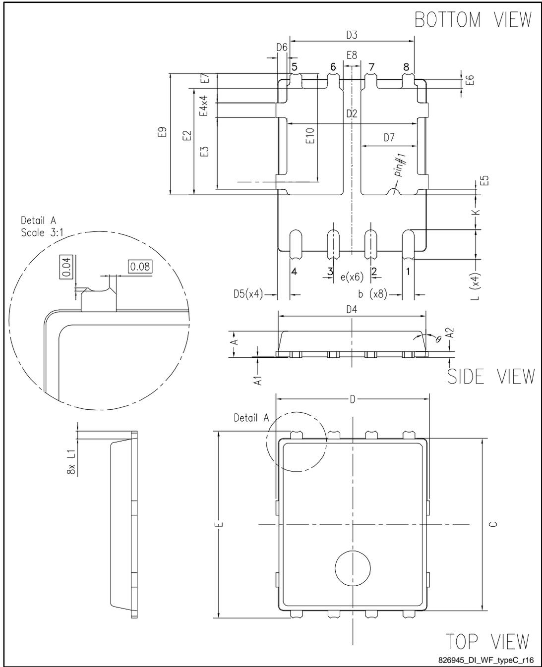
Table 8: PowerFLAT™ 5x6 double island WF type C mechanical data
