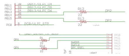
If higher file access speed is desired, a ULPI PHY (for example FUSB2805) can be added on USB1 port, which will change the USB interface to High-Speed bus (480Mbps).
