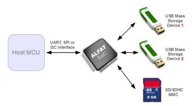
The Host MCU controls ALFAT through simple commands sent through UART (serial), SPI or I2C. The commands give the host MCU the ability to access files on the storage media. With ALFAT, file access rate can reach 4000 KBytes/sec.
