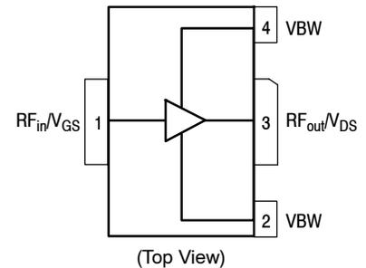
**Figure 1. Pin Connections**
