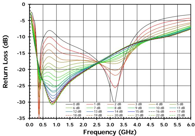
Figure 10. Output Return Loss for DSA1 Settings
