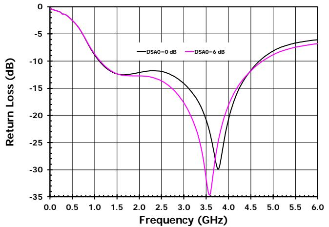
Figure 9. Input Return Loss for DSA1 Settings
