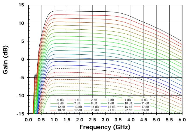
Figure 5. Gain vs. Frequency for DSA2 Settings
