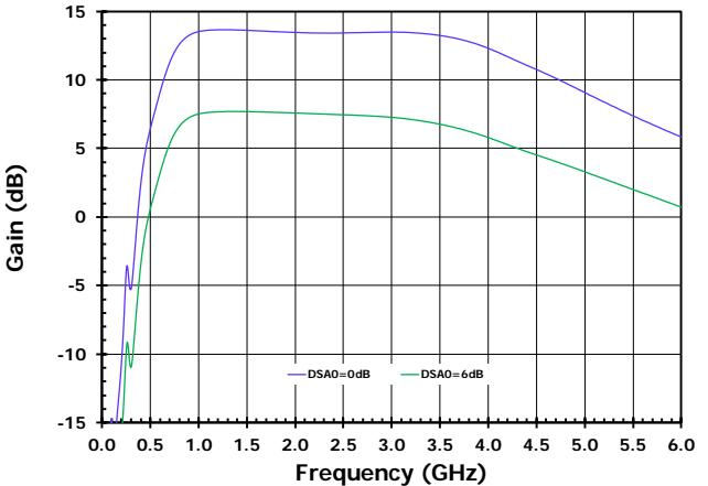
Figure 4. Gain vs. Frequency for DSA1 Settings
