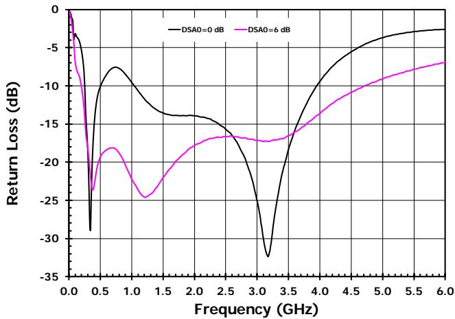
Figure 8. Output Return Loss for DSA0 Settings
