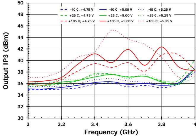
Figure 27. OIP3 vs. Frequency with
