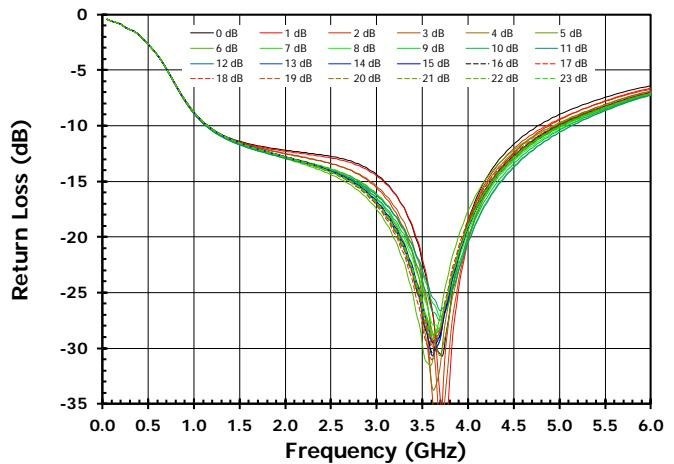
Figure 11. Input Return Loss for DSA2 Settings
