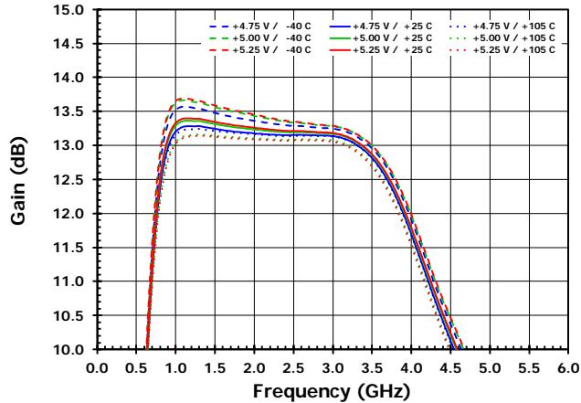
Figure 3. Gain vs. Frequency for DSA0 Settings
