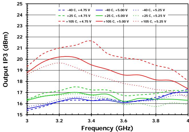
Figure 29. OIP3 vs. Frequency with
