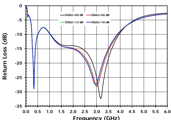
Figure 12. Output Return Loss for DSA2 Settings
