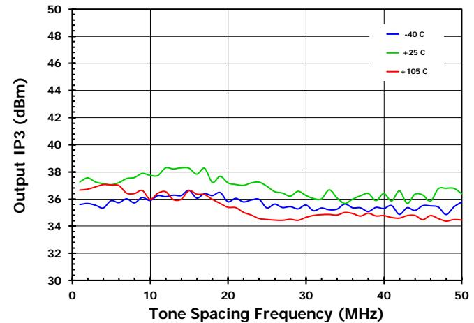
Figure 30. Wideband OIP2 vs. Frequency with  $P_{OUT} = -10\text{dBm/Tone}$
