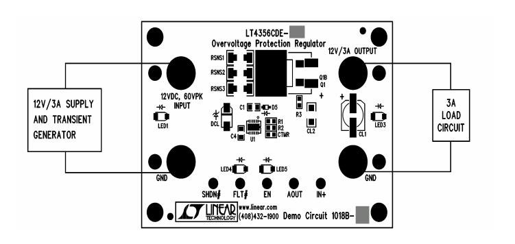
Figure 1: Proper Measurement Equipment Setup
