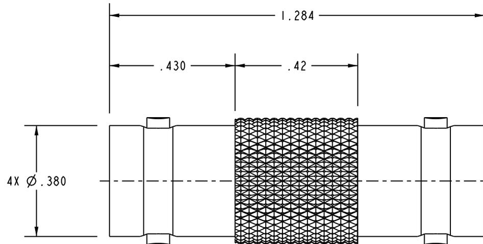
2. WITHIN SERIES FEMALE BNC FEEDTHRU ADAPTER, 50 $\Omega$  AND 75 $\Omega$  VERSIONS
