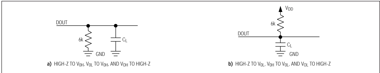
Figure 1. Load Circuits for Enable and Disable Time
