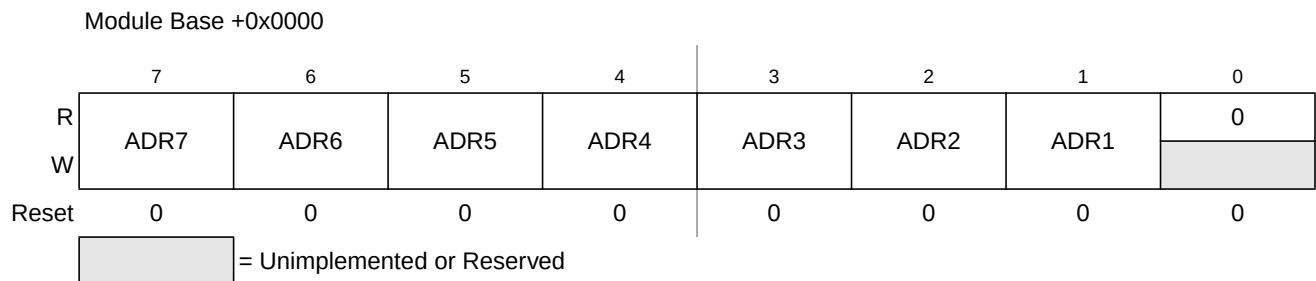
Figure 12-3. IIC Bus Address Register (IBAD)
