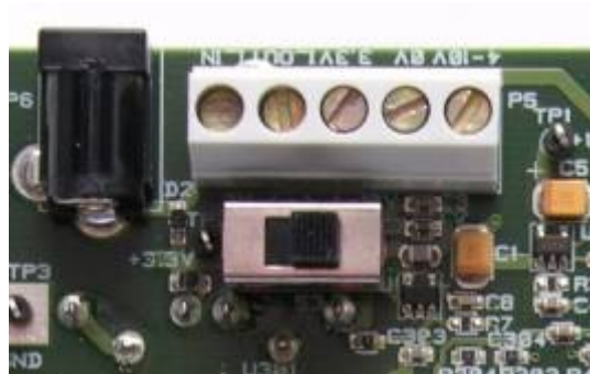
Figure 4: Power switch setting
