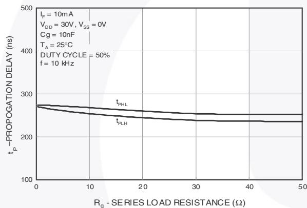
Fig. 17 Propagation Delay vs. Series Load Resistance
