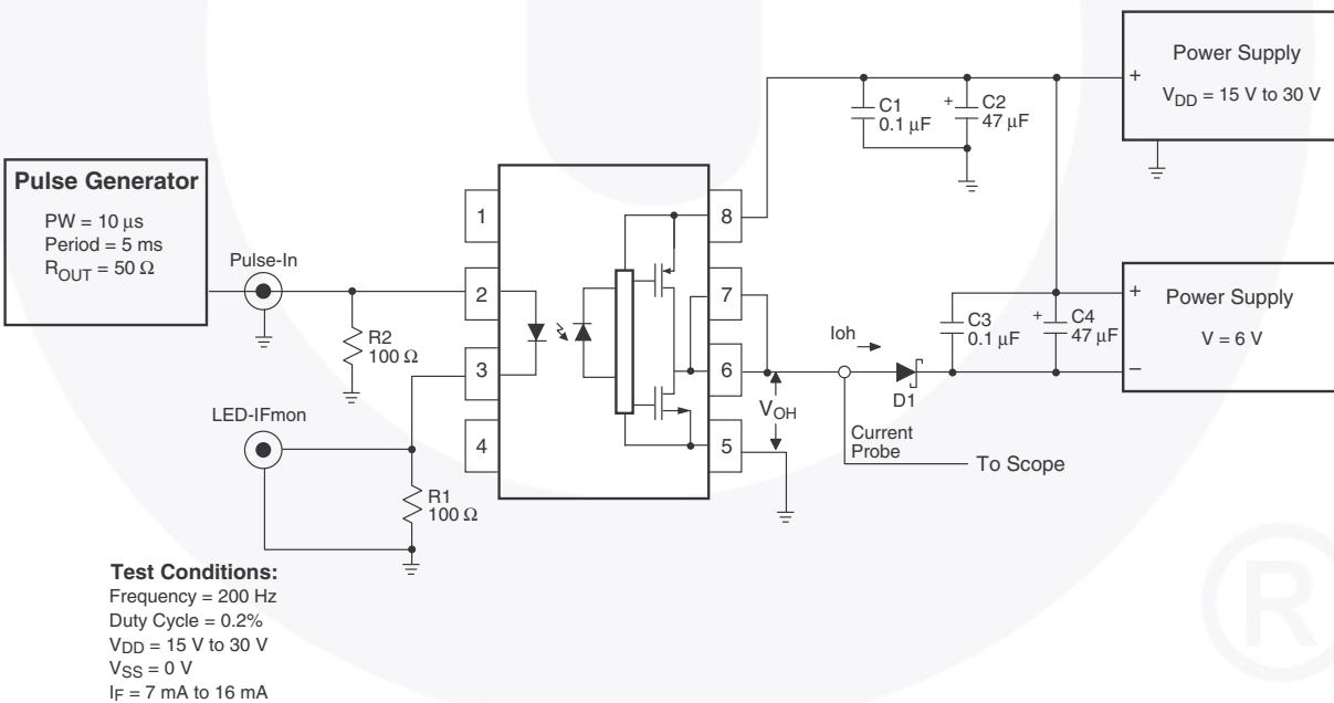
Figure 23. I<sub>OH</sub> Test Circuit
