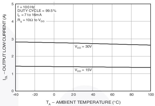
Fig. 10 Output Low Current vs. Ambient Temperature
