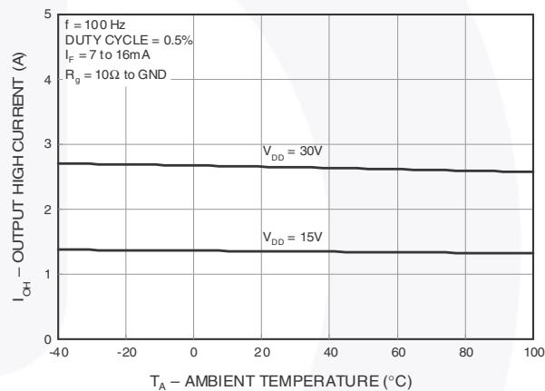
Fig. 6 Output High Current vs. Ambient Temperature
