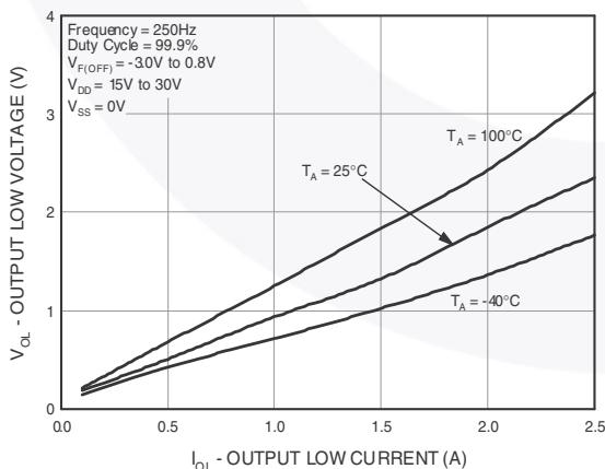
Fig. 7 Output Low Voltage vs. Output Low Current
