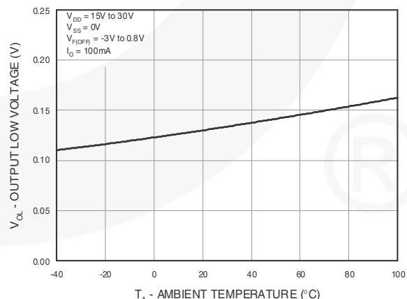
Fig. 8 Output Low Voltage vs. Ambient Temperature
