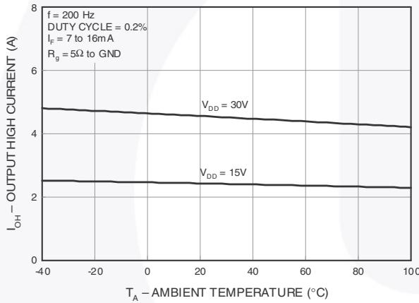
Fig. 5 Output High Current vs. Ambient Temperature
