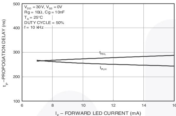
Fig. 15 Propagation Delay vs. LED Forward Current
