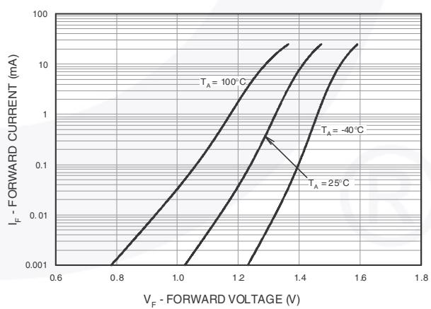
Fig. 20 Input Forward Current vs. Forward Voltage
