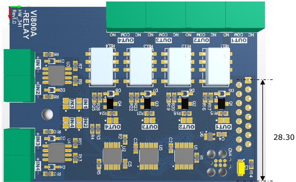
**Figure 3-2 - VI800A-RELAY module PCB Top view**
