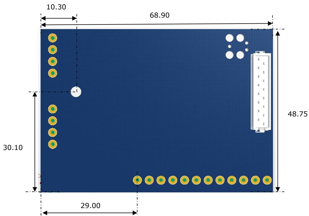
**Figure 3-3 - VI800A-RELAY module PCB Bottom view**
