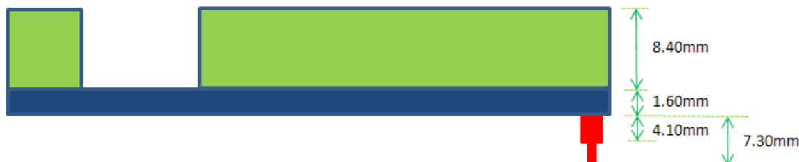
Figure 3-4 - VI800A-RELAY module PCB Side view
