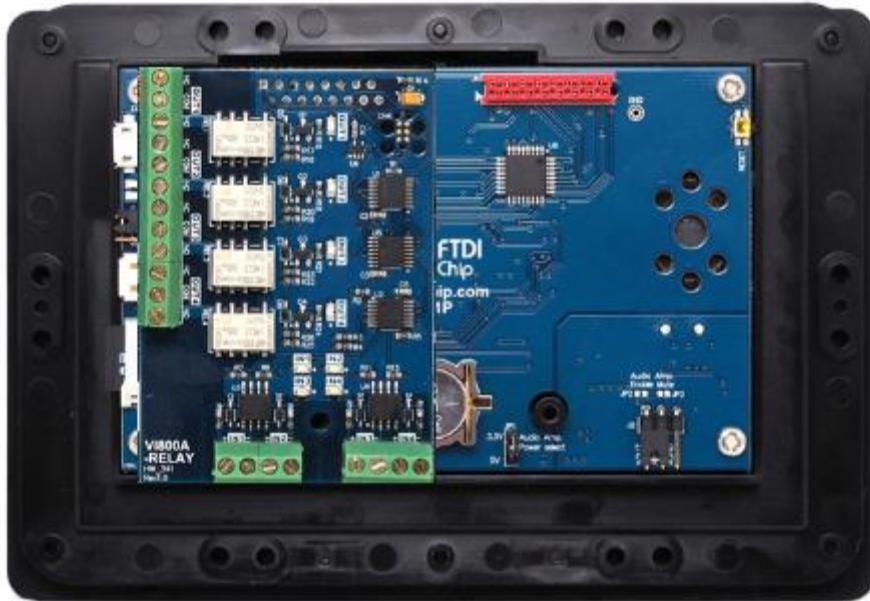
**Figure 5-1 - VI800A-RELAY module connected to VM800P Plus module**
