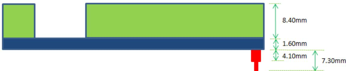
**Figure 3-4 - VI800A-RELAY module PCB Side view**
