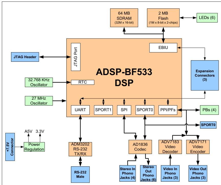
Figure 2-1. System Architecture
