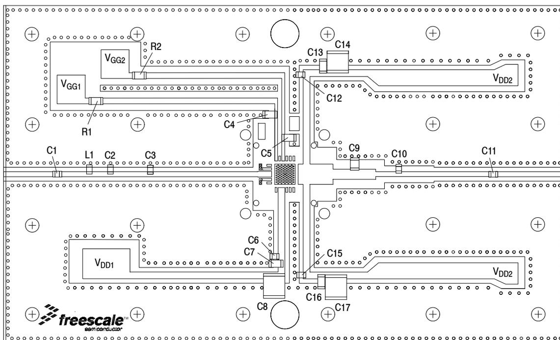
Figure 14. MMRF2006NT1 Test Circuit Component Layout — 1800 MHz
