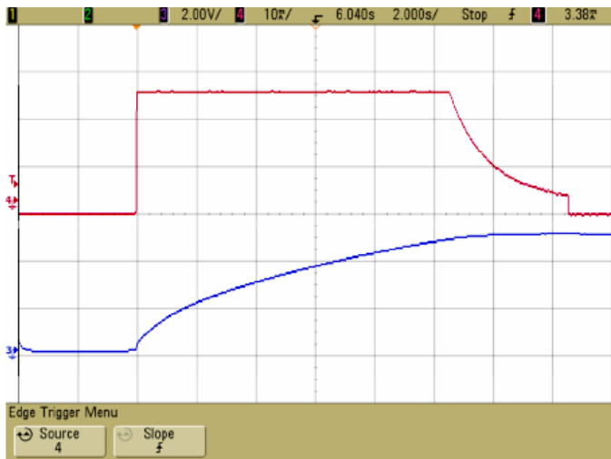
Figure 3. Charging Mode, V_{SYS} 2.5V, Input Current Set to 0.5A, Ch 4 (Red) Input Current, 200mA/DIV, Ch3 (Blue) VCAP Voltage
