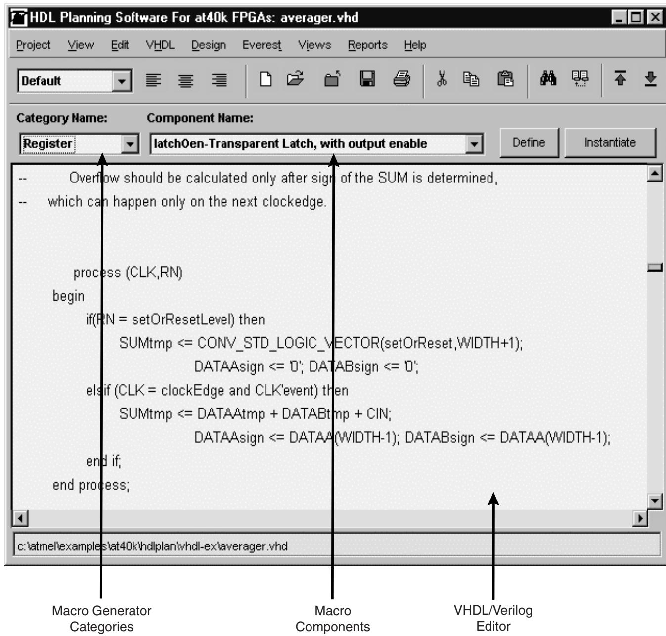
**Figure 3.** Macro Generator
