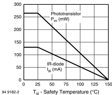
Fig. 1 - Derating Diagram
