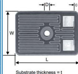
Fixing hole is located centrally except on WSHR1/2 where the dimension from the edge by the terminations to the mounting hole centre is 16.68mm.
