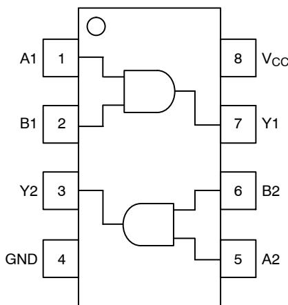
Figure 1. Pinout
