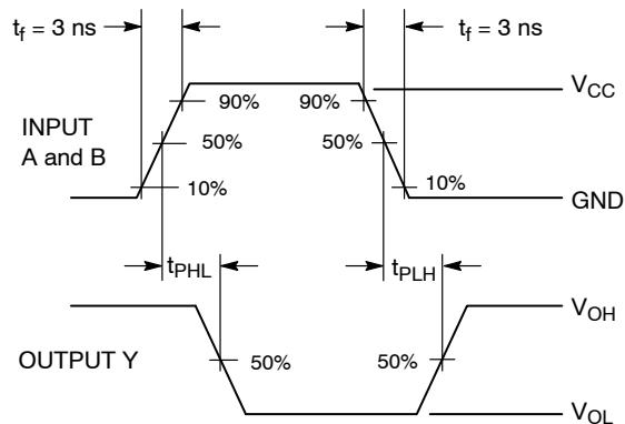
**Figure 3. Switching Waveform**
