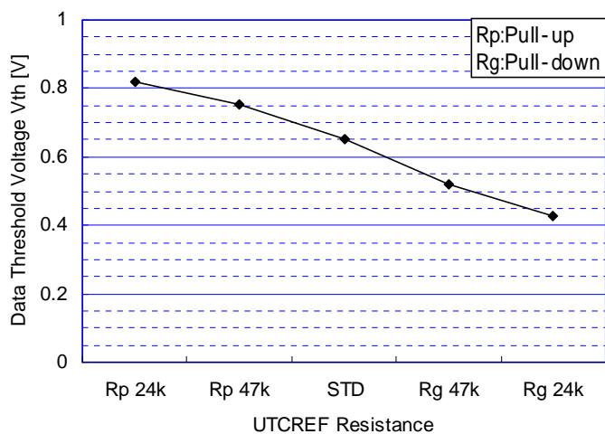
Data Threshold Voltage vs. UTCREF Resistance
