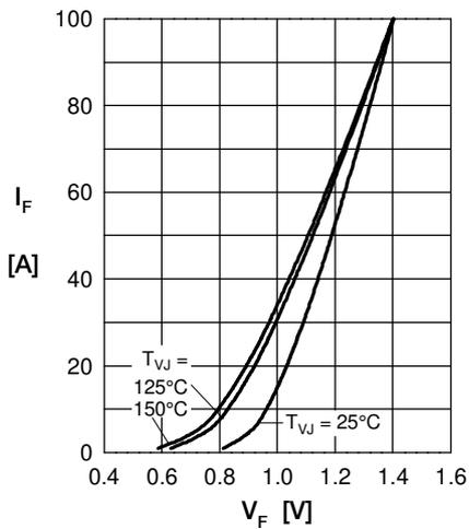
Fig. 1 Forward current vs. voltage drop per diode
