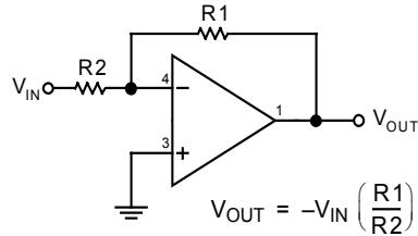
**Figure 2. Inverting Amplifier**
