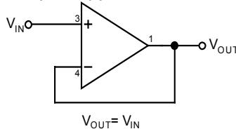
**Figure 1. Voltage Buffer**
