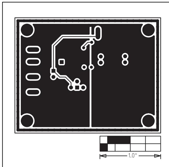
Figure 6. MAX9705B EV Kit PC Board Layout—GND Layer 3
