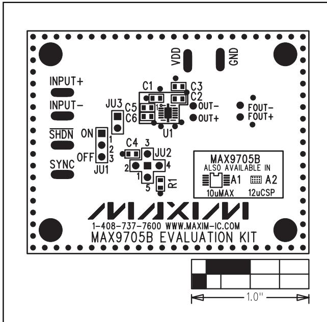
Figure 3. MAX9705B EV Kit Component Placement Guide—Component Side
