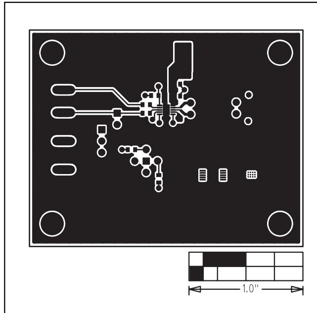
Figure 4. MAX9705B EV Kit PC Board Layout—Component Side
