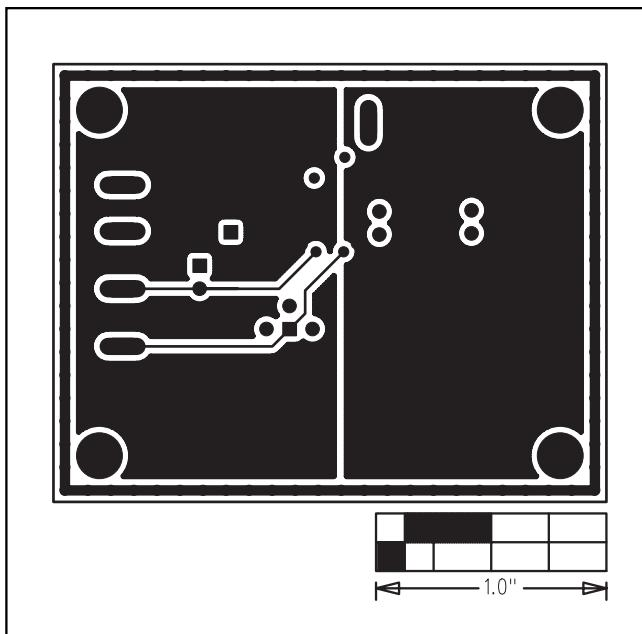
Figure 5. MAX9705B EV Kit PC Board Layout—GND Layer 2
