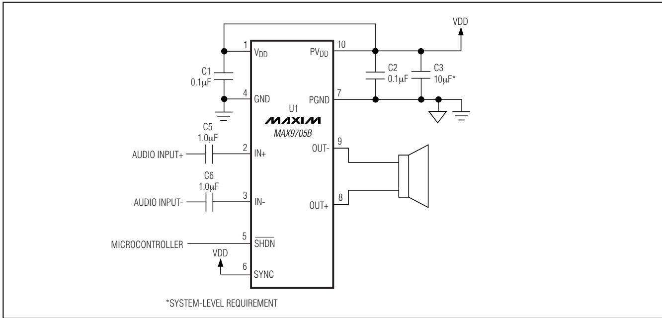
Figure 1. MAX9705B EV Kit Customer Design Schematic
