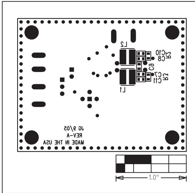
Figure 8. MAX9705B EV Kit Component Placement Guide—
