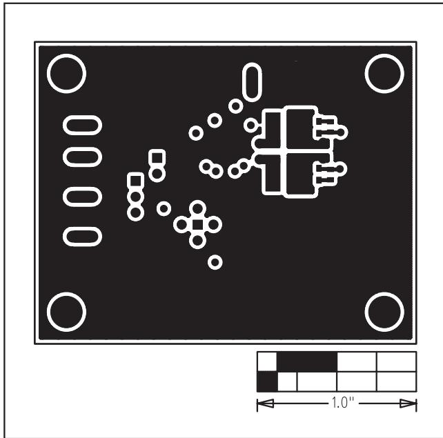
Figure 7. MAX9705B EV Kit PC Board Layout—Solder Side
