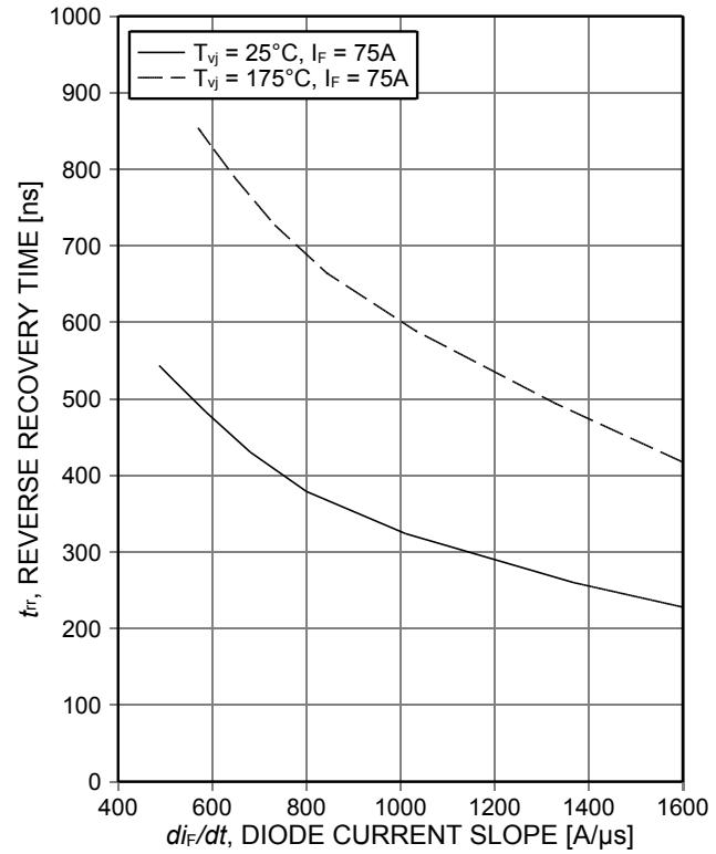
Figure 22. Typical reverse recovery time as a function of diode current slope
