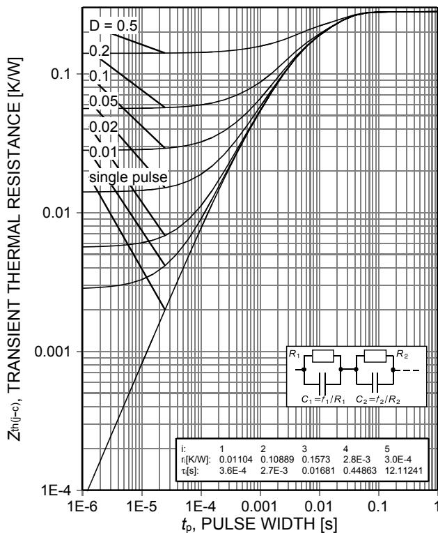
Figure 21. Diode transient thermal impedance as a function of pulse width
