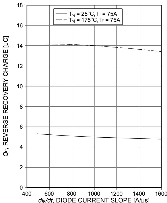
Figure 23. Typical reverse recovery charge as a function of diode current slope
