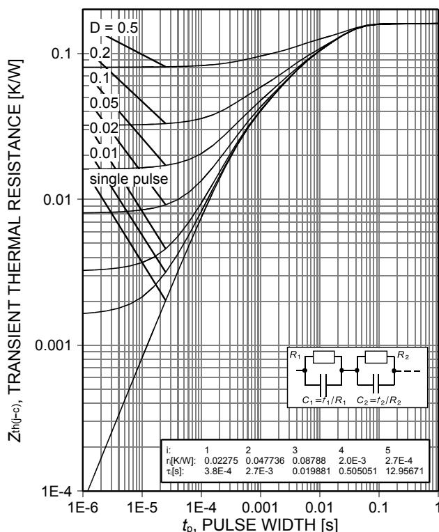
Figure 20. IGBT transient thermal resistance
