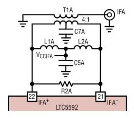
Figure 1. IF Output with Bandpass Matching
