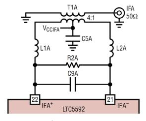
Figure 3. IF Output with Lowpass Matching
