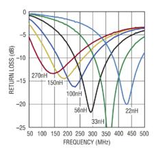
Figure 2. IF Output Return Loss with Bandpass Matching
