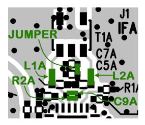
Figure 4. IF Output with Lowpass Matching
