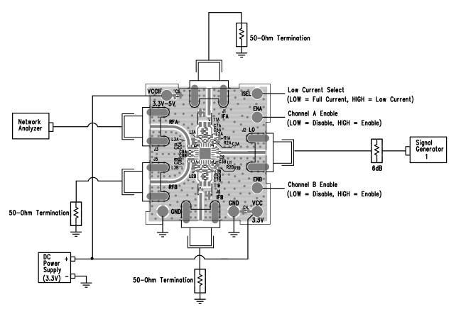
Figure 5. Proper Equipment Setup for Return Loss Measurements
