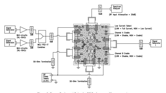
Figure 6. Proper Equipment Setup for RF Performance Measurements
