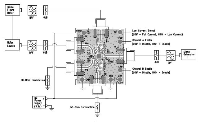
Figure 7. Proper Equipment Setup for Noise Figure Measurement
