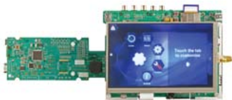
QNX® Software Systems Neutrino® RTOS and Aviate® Middleware Suite on the MCIMX35LPDK
