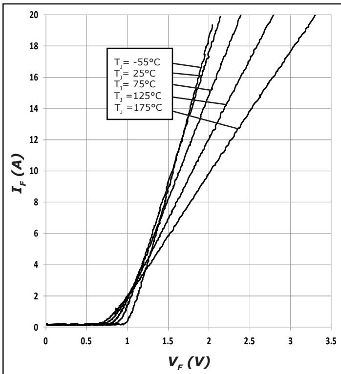
Figure 1. Forward Characteristics
