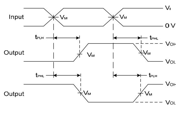
Figure 1. Load Circuit and Voltage Waveforms
