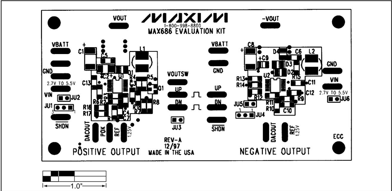
Figure 2. MAX686 EV Kit Component Placement Guide
