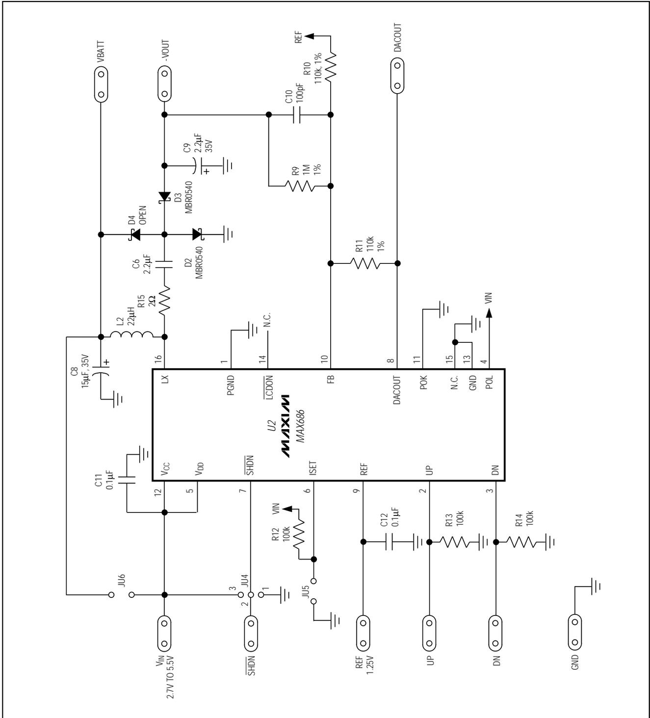
Figure 1b. MAX686 EV Kit Negative Output Schematic
