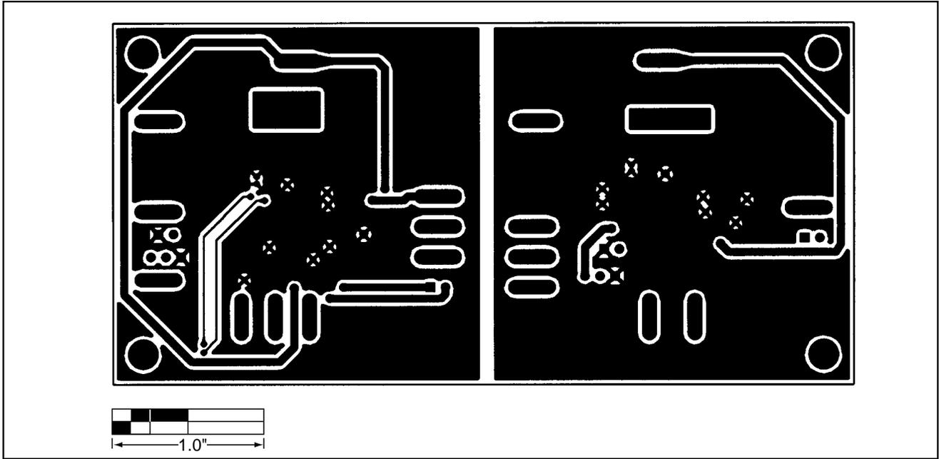
Figure 4. MAX686 EV Kit PC Board Layout—Solder Side
