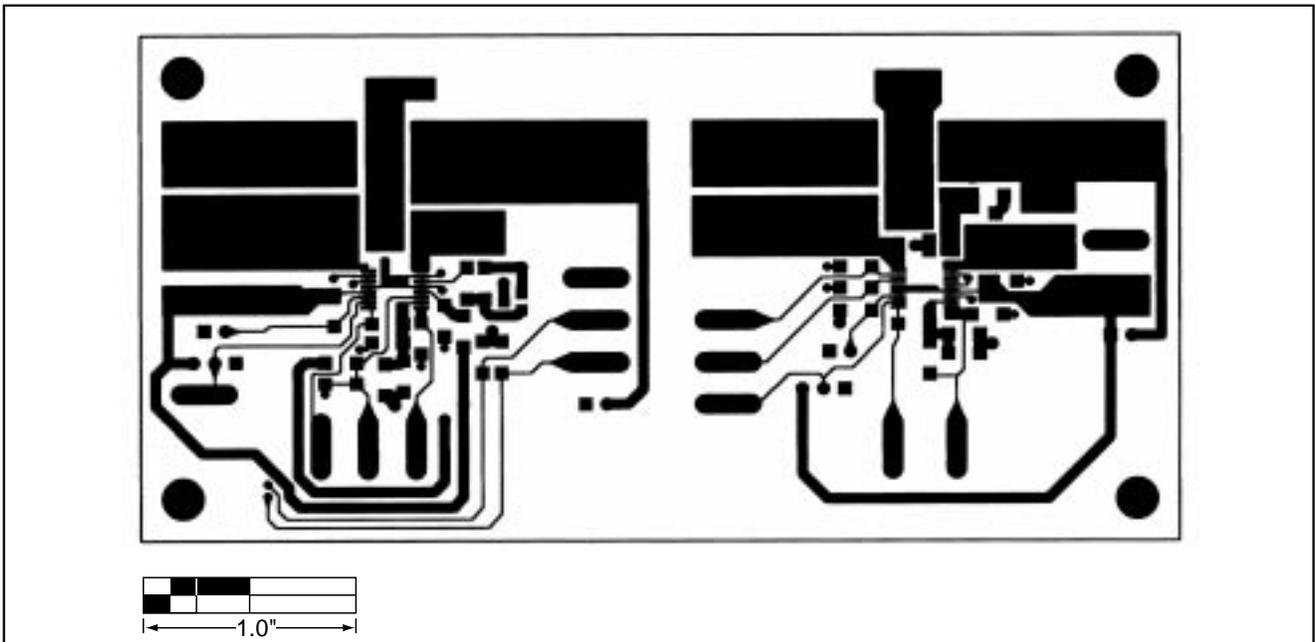
Figure 3. MAX686 EV Kit PC Board Layout—Component Side
