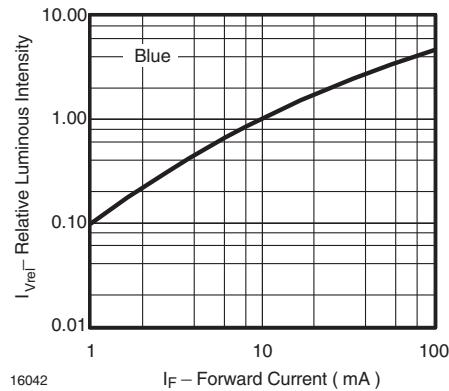
Figure 8. Relative Luminous Flux vs. Forward Current
