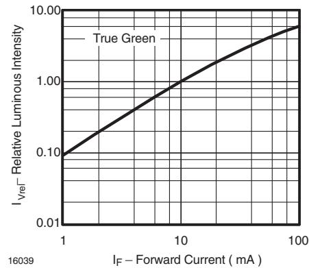
Figure 11. Relative Luminous Flux vs. Forward Current
