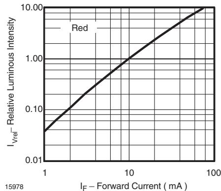
Figure 7. Relative Luminous Flux vs. Forward Current
