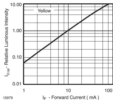
Figure 10. Relative Luminous Flux vs. Forward Current
