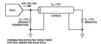
Figure 5a. Analog Output Termination for RS-343A
