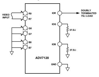
Figure 6. Input and Output Connections for Stand-Alone Gray Scale or Composite Video
