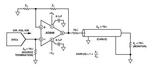
Figure 7. AD848 As an Output Buffer
