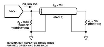
Figure 5b. Analog Output Termination for RS-170
