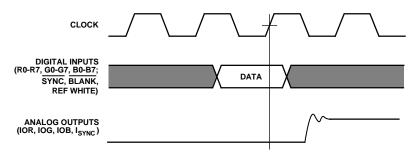
Figure 2. Video Data Input/Output
