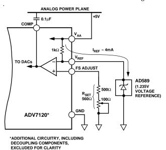
Figure 4. Reference Circuit
