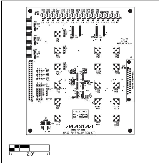
Figure 2. MAX3170 EV Kit Component Placement Guide—
