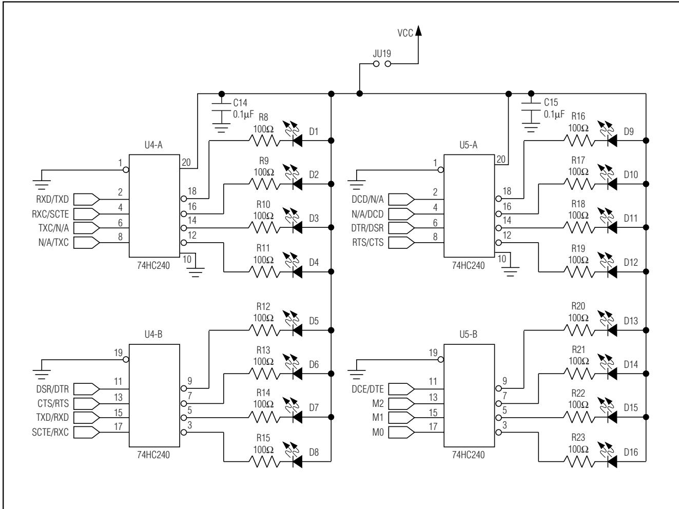
Figure 1. MAX3170 EV Kit Schematic (Sheet 2 of 2)
