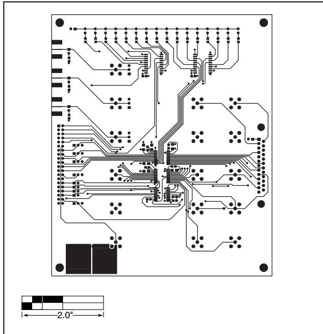
Figure 3. MAX3170 EV Kit Component Placement Guide—
