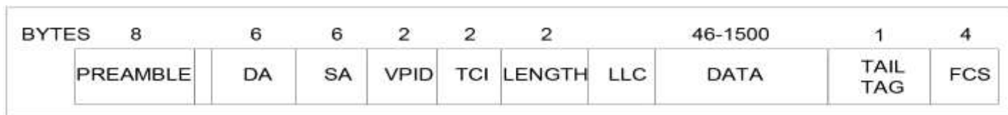
Figure 13. Tail Tag Frame Format
