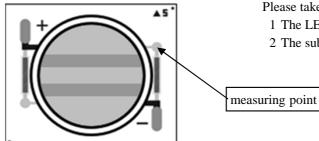
Please take note of the following, when measuring case temperature. 1 The LED device mounting surface should be flat/plain surface. 2 The substrate surface temperature should be uniform.
