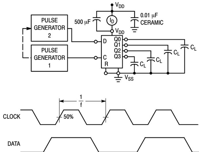
Figure 1. Power Dissipation Test Circuit and Waveform
