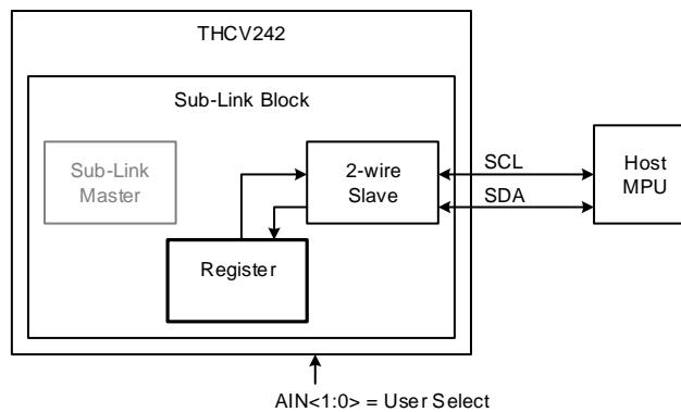
**Figure 3.** Host to THCV242 local register access configuration
