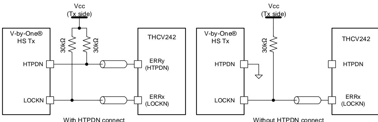
**Figure 2.** Physical wire connection for wired Hot-plug and Lock detect scheme
