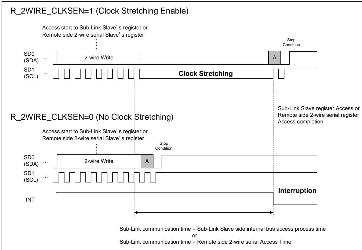
**Figure 8.** Sub-Link Master 2-wire slave clock stretching operation
