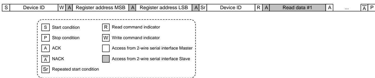
**Figure 5.** 2-wire serial I/F read to THCV242 local register protocol
