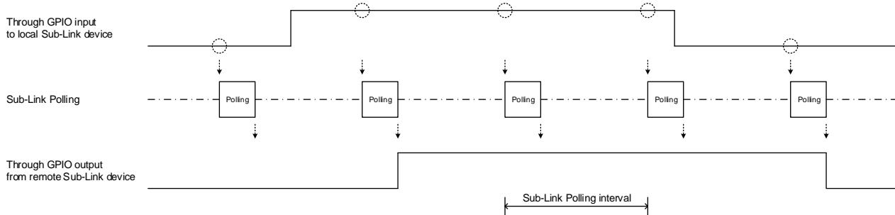
**Figure 11.** Through GPIO bridge sampling
