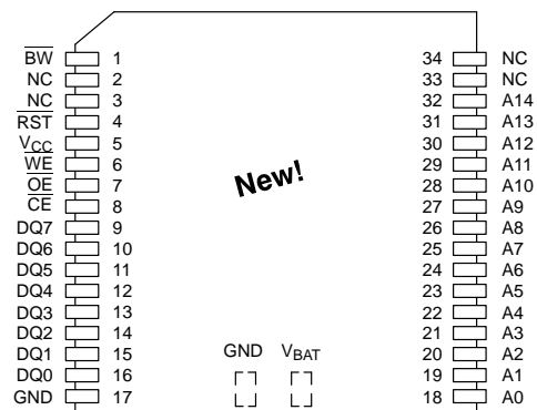
34-PIN POWERCAP MODULE (PCM) (USES DS9034PC POWERCAP)
