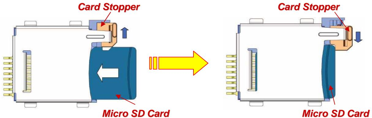
During insertion process, micro SD card pushes aside the self-retractable card stopper. Once micro SD card is fully inserted, the card stopper will return to original position by internal spring action and lock the micro SD card into position for secured connection.
